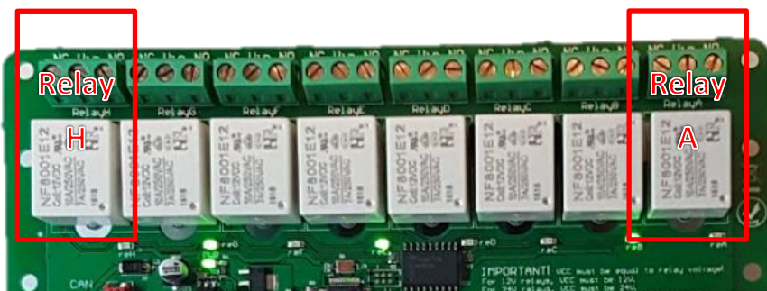
Figure 2: Relay naming - relay outputs are marked with letters A to H in order as indicated
